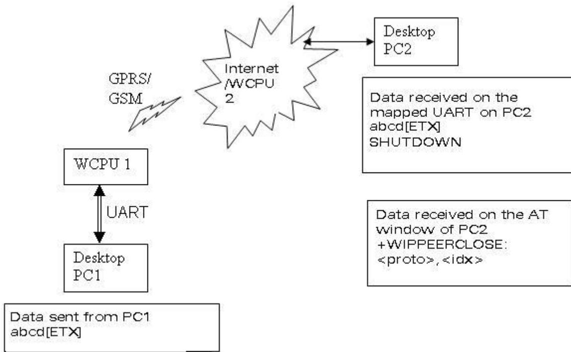
In the schematic above, a TCP socket is connected. On the transmitting side, data and [ETX] is sent (use case: Desktop PC1 is a WISMO® which sends data to PC2 which is either a PC or also a WISMO®), and the data is received on PC2 and the [ETX] character shuts down the socket on the transmitting side and displays a message “[CR][LF]SHUTDOWN[CR][LF]” on the UART of PC2.
