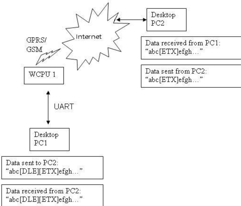
The schematic above explains how [DLE] characters – which have a special meaning in the firmware – are handled on the WISMO®.
