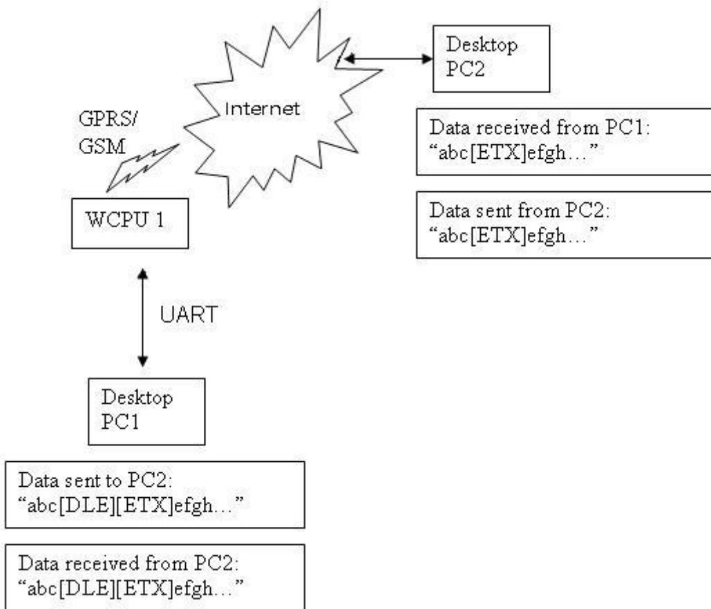
The schematic above explains how [ETX] characters – which have a special meaning in the firmware – are handled on a WISMO®.
